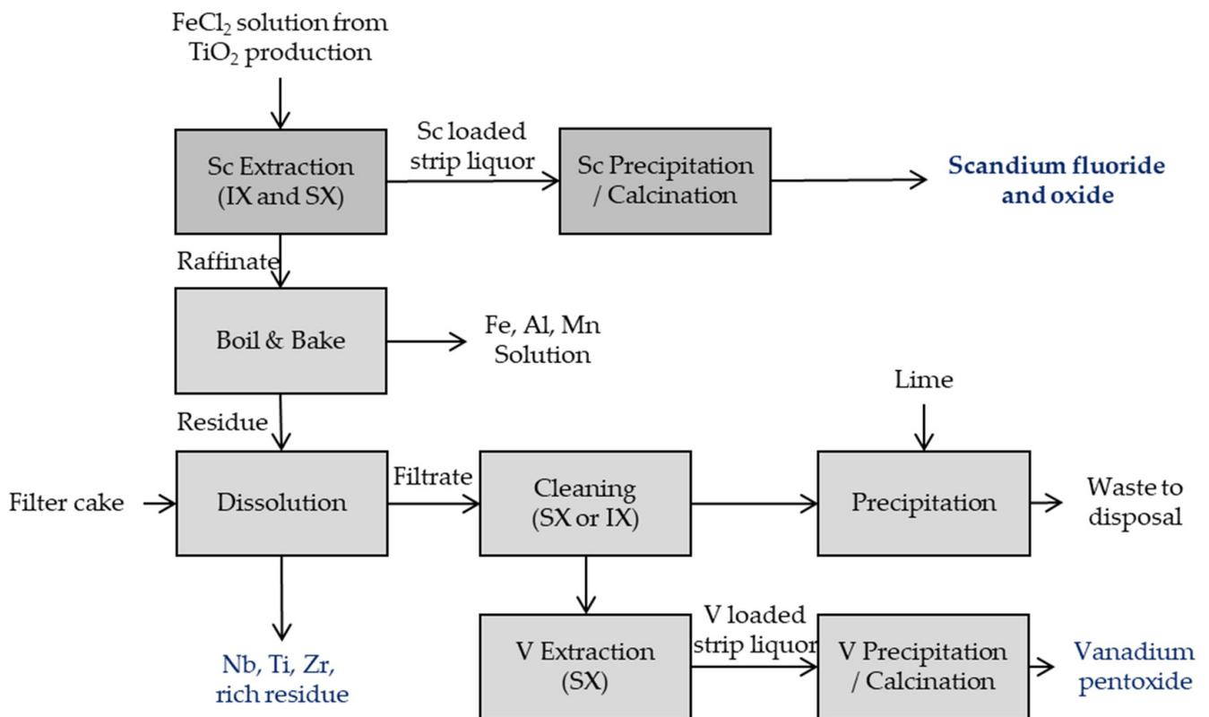
**Figure 1.** Conceptual process flow sheet of ScaVanger.
