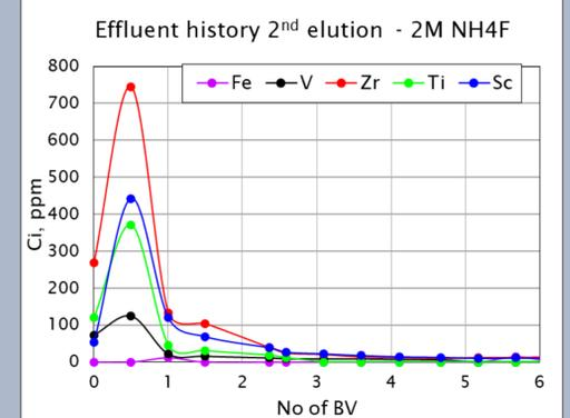
Figure 5. Fractional concentration in effluent solution during NH<sub>4</sub>F elution (ppm)
