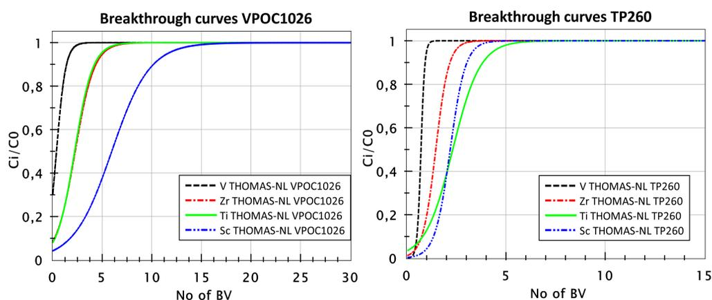
Figure 2. Breakthrough curves for metals of interest in VPOC1026 resin (2a) and TP260 (2b)
