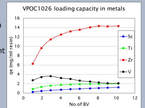
Figure 3. Loading capacity of resin, q<sub>e</sub> (mg/mL)
