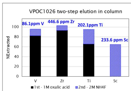
Figure 6. Overall extraction rate of Elution
