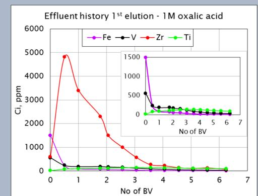
Figure 4. Fractional concentration in effluent solution during oxalic acid elution (ppm)
